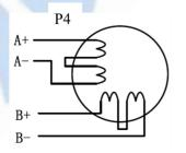
Figure 10 8-lead motor series connection
