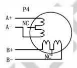
Figure 9 6-lead motor full coil connection
