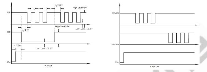
Figure 13 Sequence chart of control signals
