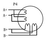
Figure 11 8-lead motor parallel connection
